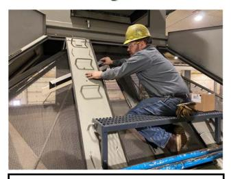
Our 80K screener also features 8 diverters that rotate & slide up/down for desired clearance to screens. These diverters spread grain to fully utilize those "Hard to Reach" corners of the screens.
