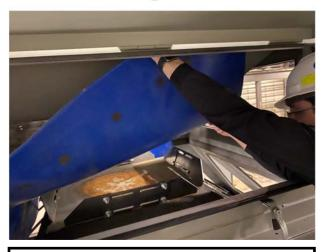
Sliding baffles direct flow to different areas of screen as well as fine tuning grain flow equally to all 4 sides of the screener.
