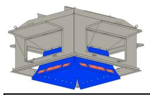
Urethane drapes slow the grain down to provide a consistent even flow of grain over the screening surface. Weights can be added to direct flow evenly over screens as well as equally to all 4 sides of the screener.
