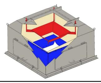
It is almost impossible to design up-line spouting to provide equal grain flow to all 4 sides of the screener. This adjustable basket directs incoming grain for even distribution to the screener, it also acts as a flow retarder to slow the grain down as it enters the screener.
