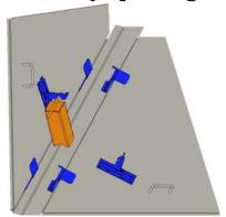
Screener doors (8) have form down lips 4 sides for a positive seal. "SELF LATCHING" brackets hold doors in the open position for safety & convenience.
