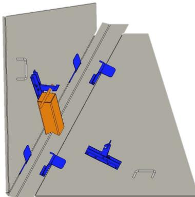
Screener doors (8) have form down lips 4 sides for a positive seal. "SELF LATCHING" brackets hold doors in the open position for safety & convenience.
