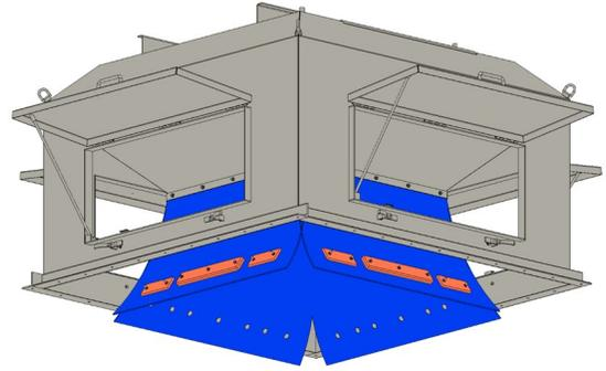
Urethane drapes slow the grain down to provide a consistent even flow of grain over the screening surface. Weights can be added to direct flow evenly over screens as well as equally to all 4 sides of the screener.
