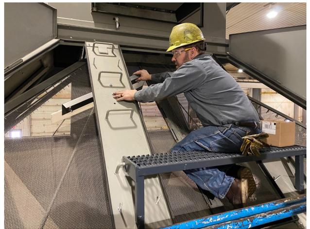
Our 80K screener also features 8 diverters that rotate & slide up/down for desired clearance to screens. These diverters spread grain to fully utilize those "Hard to Reach" corners of the screens.
