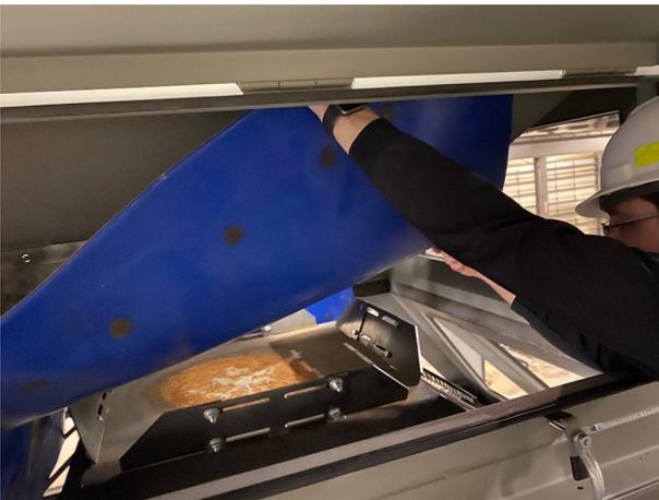
Sliding baffles direct flow to different areas of screen as well as fine tuning grain flow equally to all 4 sides of the screener.
