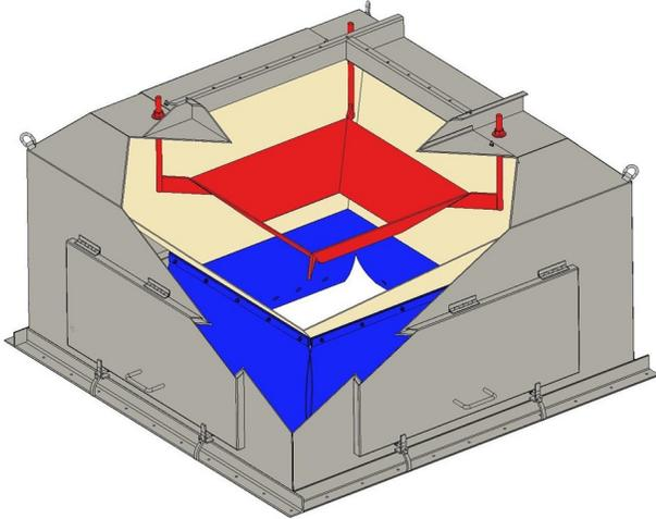
It is almost impossible to design up-line spouting to provide equal grain flow to all 4 sides of the screener. This adjustable basket directs incoming grain for even distribution to the screener, it also acts as a flow retarder to slow the grain down as it enters the screener.
