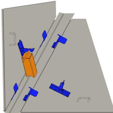
Screeners doors (8) have form down lips 4 sides for a positive seal. "SELF LATCHING" brackets hold doors in the open position for safety & convenience.
